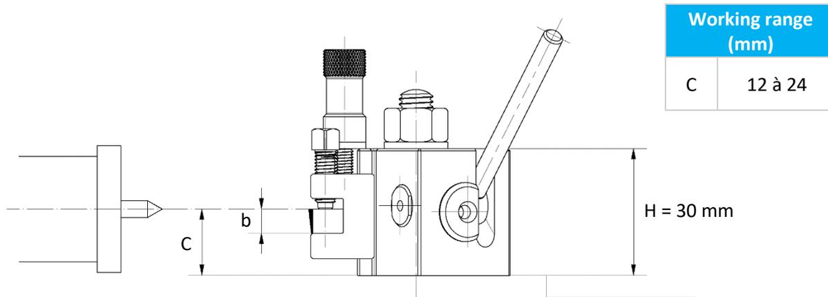
Minimum dimension C for tool bits or blades of height b (mm)
